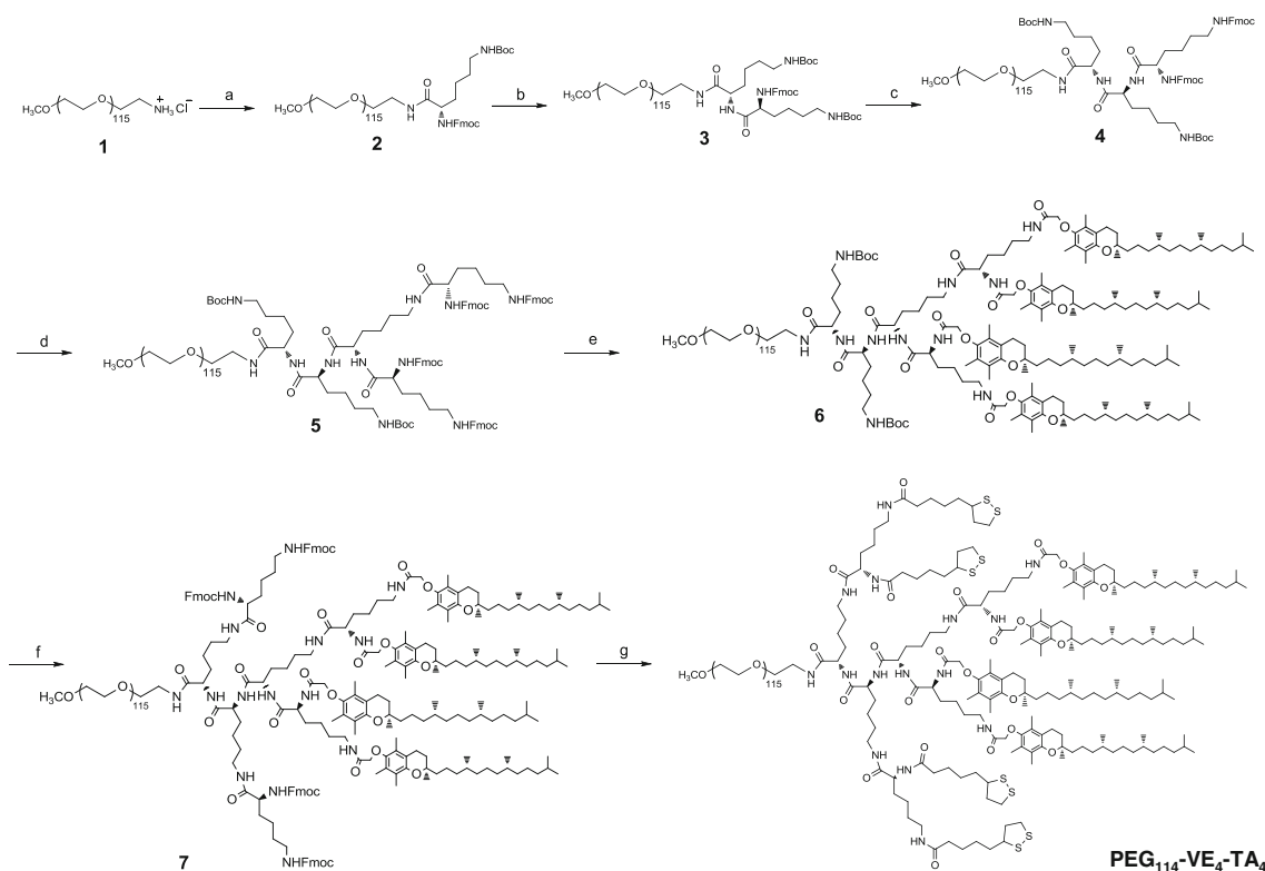
Scheme 1 Synthetic route of PEG 114 -VE 4 -TA 4 . Reagents and condition: a , Fmoc-Lys(Bos)-OH, DIC, HOBT, DIEA, DMF, r.t, 6 h. b , i, 20% Piperidine in DMF, r.t, 2 h. ii, Fmoc-Lys(Bos)-OH, DIC, HOBT, DIEA, DMF, r.t, 6 h. c and d , i, 20% Piperidine in DMF, r.t, 2 h. ii, Fmoc-Lys(Fmoc)-OH, DIC, HOBT, DIEA, DMF, r.t, 6 h. e , i, 20% Piperidine in DMF, r.t, 2 h. ii, \alpha -tocopheryloxyacetic acid, DIC, NHS, DIEA, DMF, r.t, overnight. f , i, 50% TFA in CHCl 3 , r.t, 1 h. ii, Fmoc-Lys(Fmoc)-OH, DIC, HOBT, DIEA, DMF, r.t, 6 h. g , i, 20% Piperidine in DMF, r.t, 2 h. ii, lipoic acid, DIC, NHS, DMF, r.t, overnight
